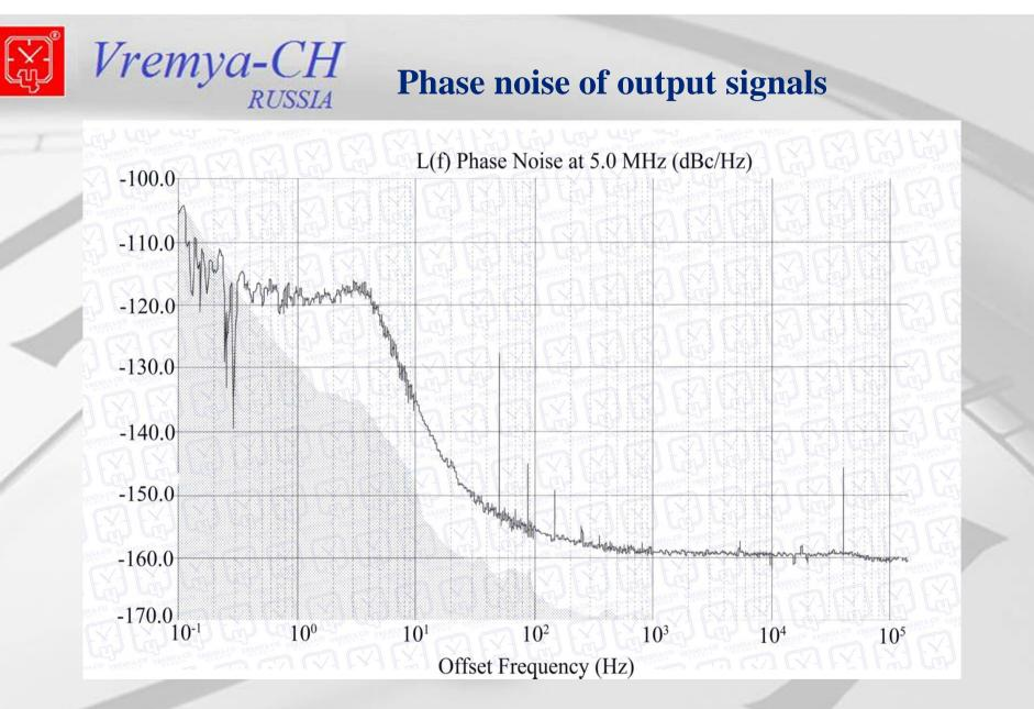
Modulation frequency's spurious components are suppressed up to the -145dBc level
