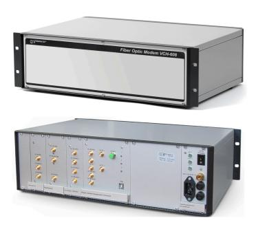
Fiber-optic modem VCH-608 is designed for receiving and transmitting signals of atomic clocks through a fiber optic communication line (FOCL).
